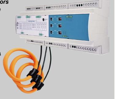
The CAL101rogo-3 is a ready install kit for application where space is insufficient for conventional current transformers. The 5A outputs is useful for direct connexion with standard measure devices (counter, wattmeter, threshold relays, ...)
