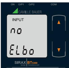
Pressing the “**Down**” key will enter the “Selection of Elbow function of Input edit” mode and scroll the value between yes and no.
