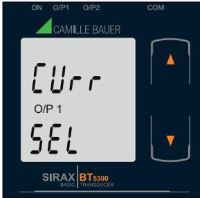
Pressing the “
