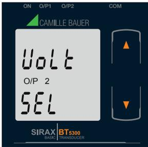
Pressing the “
