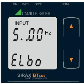
Enter New / Change Elbow value of the Input, first digit entered, prompting for second digit. (\*Denotes that digit will be flashing).
