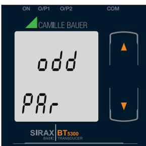
Pressing the “ Down” key will enter the “Parity & stop bit edit” mode and scroll the value through
