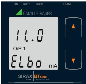
Enter New / Change Elbow value of the Output 1, second digit entered, prompting for third digit. (\*Denotes that digit will be flashing).
