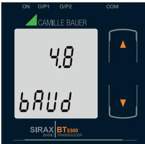
This screen allows the user to set Baud Rate of RS 485 port. The values displayed on screen are in kbaud.
