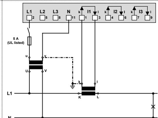
**Three wire system, balanced load, phase shift**
