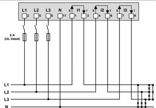
If current  $I_N$  or voltage  $U_{NE}$  does not need to be measured, connection of IN or PE can be omitted.
