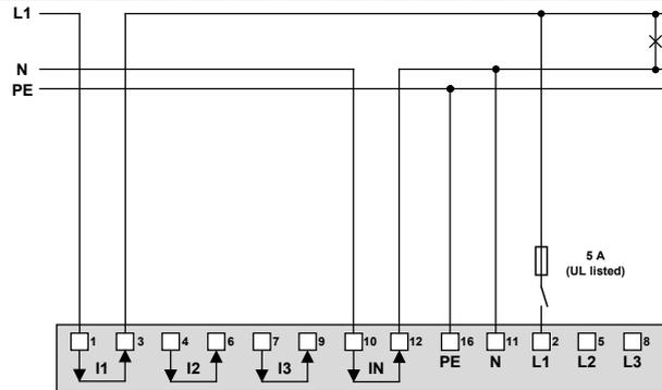
If current  $I_N$  or voltage  $U_{NE}$  does not need to be measured, connection of IN or PE can be omitted.
