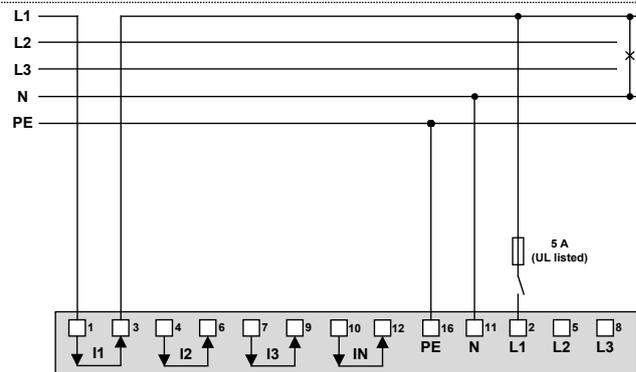
If voltage  $U_{NE}$  does not need to be measured, connection of PE can be omitted. PE is not available for AM2000.
