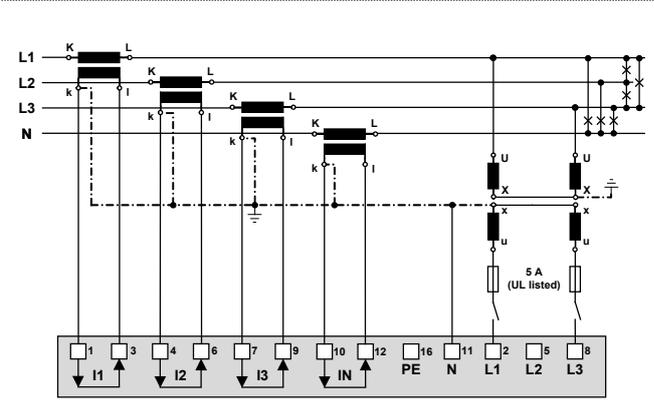
If current  $I_N$  does not need to be measured, the corresponding transformer can be omitted. IN is not available for the AM2000.
