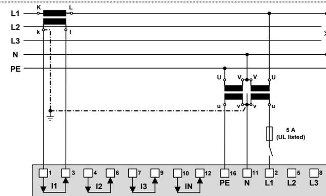
If voltage  $U_{NE}$  does not need to be measured, the corresponding transformer can be omitted. PE is not available for AM2000.
