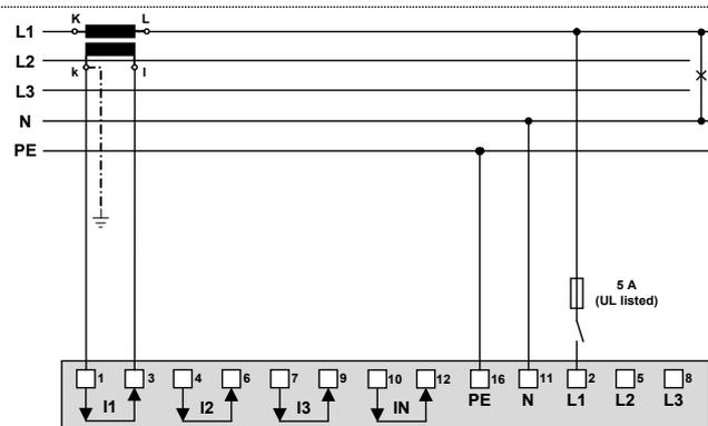
If voltage  $U_{NE}$  does not need to be measured, connection of PE can be omitted. PE is not available for AM2000.
