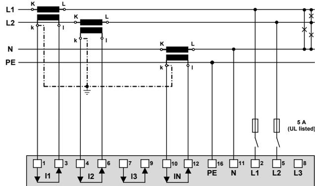
If current  $I_N$  does not need to be measured, the corresponding transformer can be omitted. If voltage  $U_{NE}$  does not need to be measured, connection of PE can be omitted.
