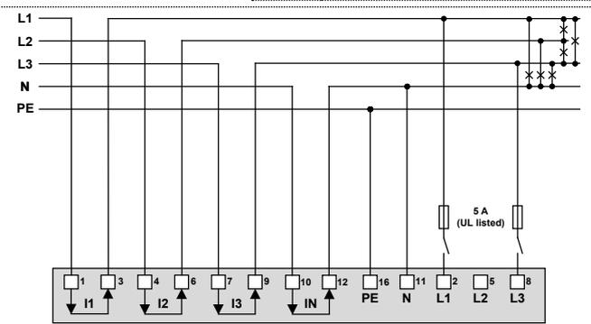
If current  $I_N$  or voltage  $U_{NE}$  does not need to be measured, connection of IN or PE can be omitted.
