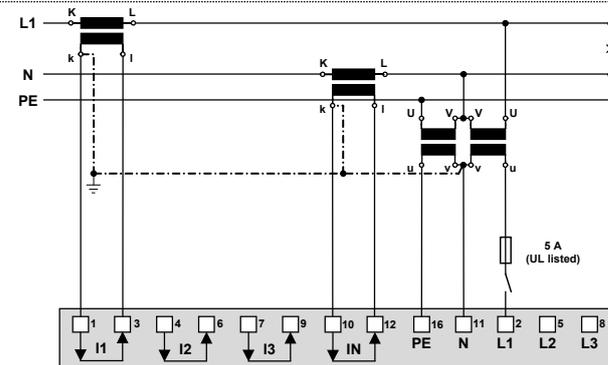
If current  $I_N$  or voltage  $U_{NE}$  does not need to be measured, the corresponding transformers can be omitted.
