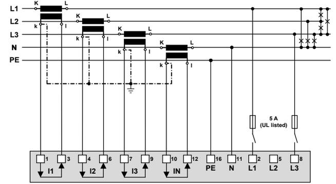
If current  $I_N$  does not need to be measured, the corresponding transformer can be omitted. If voltage  $U_{NE}$  does not need to be measured, connection of PE can be omitted.
