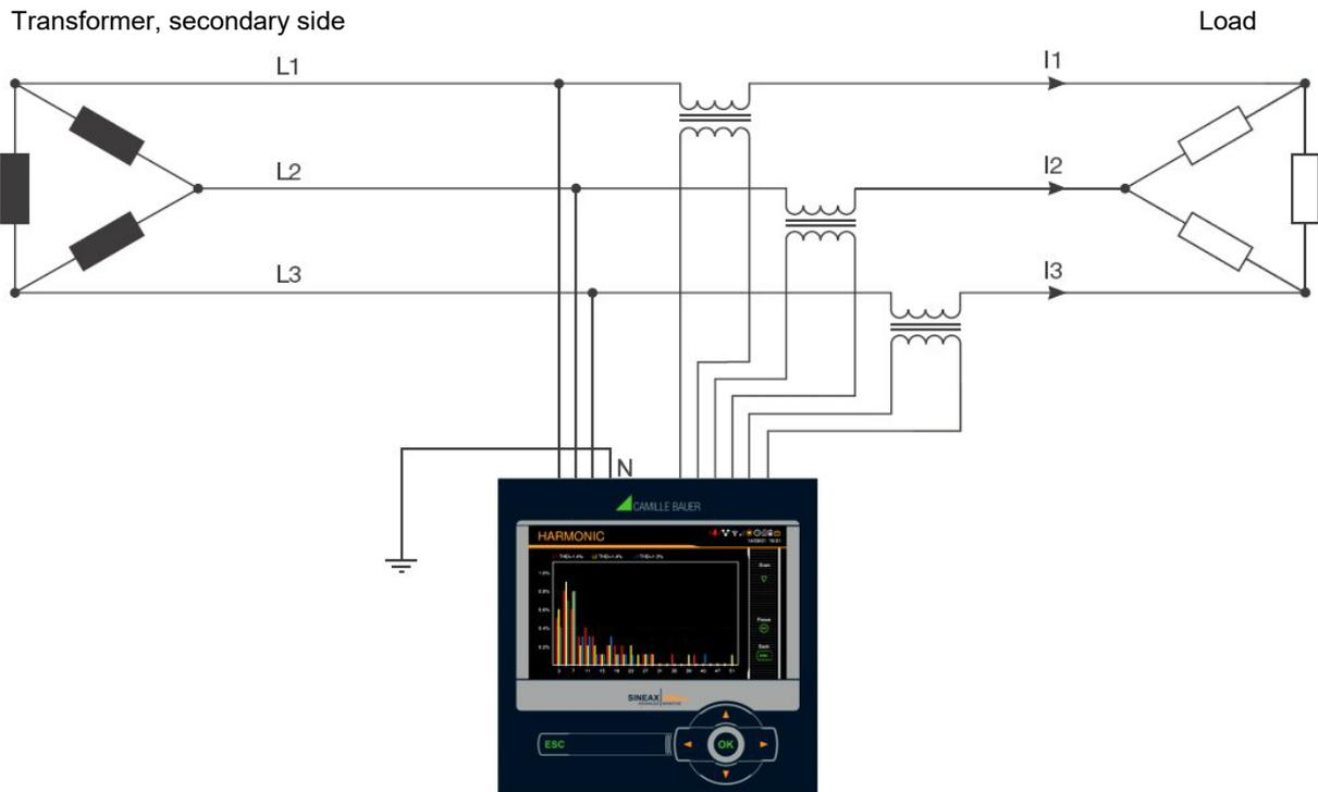
Because in case of a fault the voltage triangle formed by the three phases does not change, the voltage and current measurements as well as the system power values will still be measured and displayed correctly. Also the meters carry on to work as expected.
