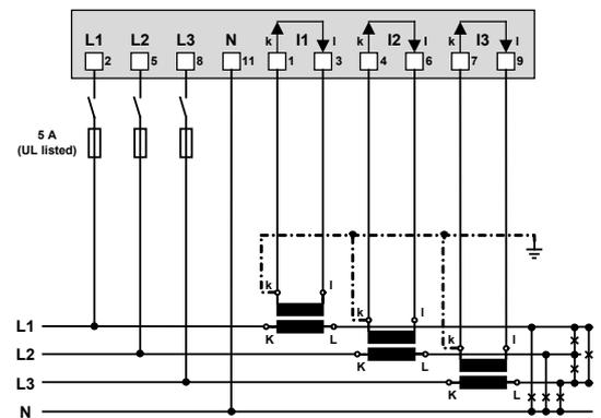
If current  $I_N$  does not need to be measured, the corresponding transformer can be omitted. If voltage  $U_{NE}$  does not need to be measured, connection of PE can be omitted.
