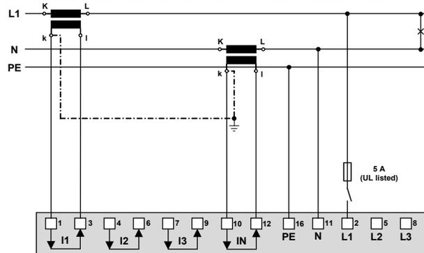
If current  $I_N$  does not need to be measured, the corresponding transformer can be omitted. If voltage  $U_{NE}$  does not need to be measured, connection of PE can be omitted.
