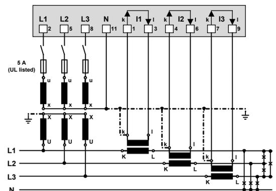
If current  $I_N$  does not need to be measured, the corresponding transformer can be omitted. IN is not available for the AM2000.
