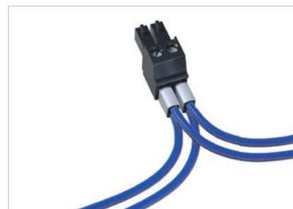
2-pole plug contact with cable connection (cable type: 2 x 0.75 mm 2 ) via twin core end sheathes
