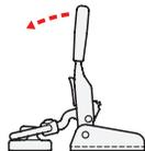
For **clamping**, lift the lever arm until the pulling latch rests against the catch.
