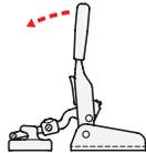
Lift the lever arm until the pulling latch is disengaged from the catch.
