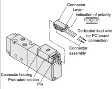
Cautions: 1. Do not pull hard on the lead wire.lt could result in defective contacts, breaking wires, etc.
