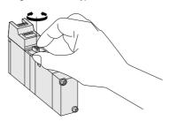
Cautions: 1. The 110 series valves are internal pilot type solenoid valves. As a result, the manual override cannot switch the main valve without air supplied from the 1(P) port.
