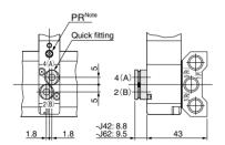
Note: PR is on the side with the 4(A), 2(B) ports.
