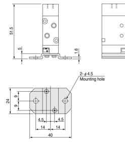
• With quick fittings: **-J42** (For  $\phi$  4 tube, 4(A), 2(B) ports with fittings)
