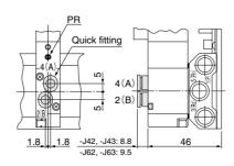
Note: PR is on the side with the 4(A), 2(B) ports.
