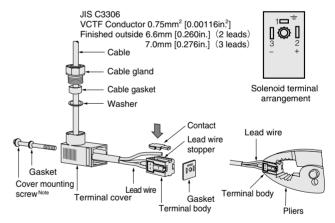
Note: The appropriate tightening torque for the cover mounting screw is 29.4N-cm {3kgf-cm} [2.6in-lbf].
