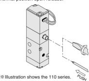
Cautions: 1. The 110 series valves are internal pilot type solenoid valves. As a result, the manual override cannot switch the main valve without air supplied from the 1(P)
