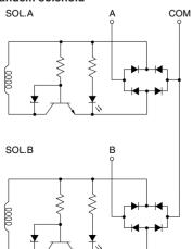
Cautions: 1. Do not apply megger between the lead wires
