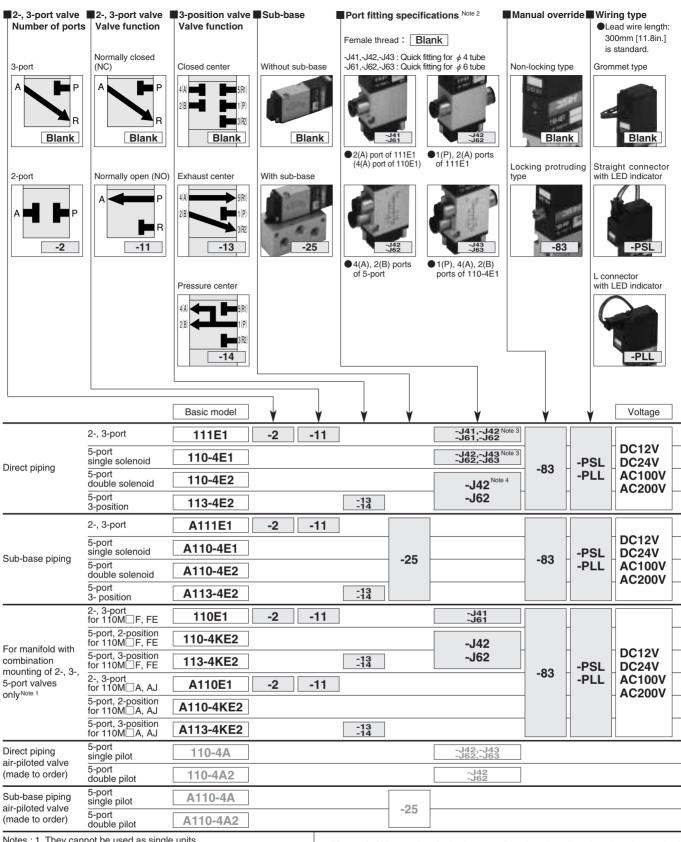
Notes : 1. They cannot be used as single units. 2. The port fittings are for  $\phi$  4: TSK4-M8M, and for  $\phi$  6:
