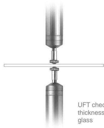
UFT checking thickness of thin glass
