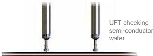
UFT checking semi-conductor wafer
