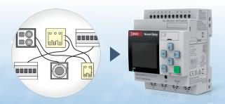
■ The FL1F is a smart solution for simplifying complex wiring, including relays, timers, and counters. It supports up to a 10A output and features a message display function.
