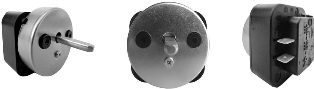
120 minute, 20 mm shaft, two sets of horizontal contacts, with bell, with "hold", mounted with two screws 2,9 x 8 mm.
