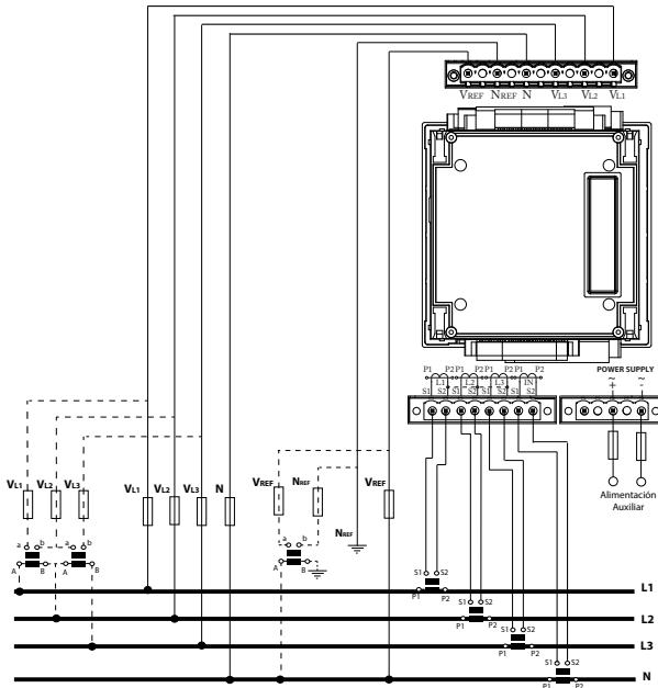
Direct phase-phase measurement with current transformers
