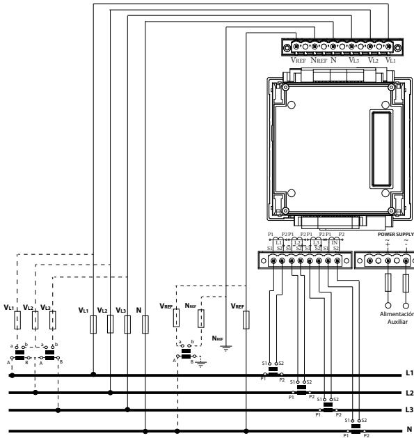
Direct phase-phase measurement with current transformers
