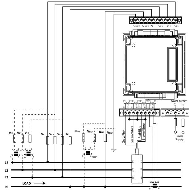
Measurement in single-phase system with or without voltage transformer
