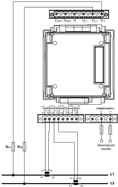
Three-phase measurement, with or without voltage transformer and MC3 type transformers (1250 mA) + MC1 for neutral current
