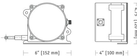
The SR1M is part of a series of rugged, low-cost, high performance string pots built for wet environments and outdoor applications. Designed for the rigors of outdoor construction equipment or the demands of a factory floor, the SR1M is the perfect low-cost solution for OEM and stocking distributors.
