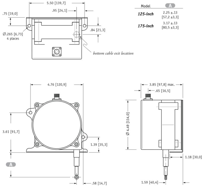
**Fig. 4 - "Rear" Cable Exit Direction**
