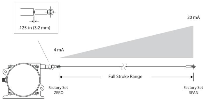
*This is for the factory setting only and the ZERO may be reprogrammed at full retraction at any time.*
