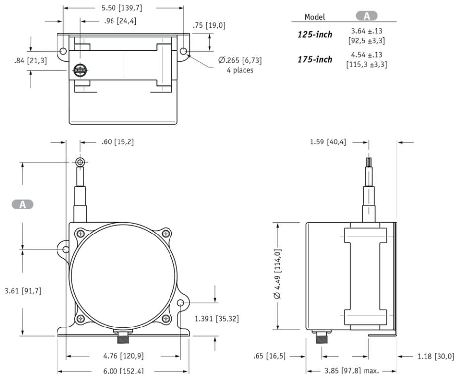
**Fig. 3 - "Down" Cable Exit Direction**
