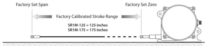
Please note that ZERO and SPAN points can be set independently. You can set one without setting the other. This operation must be performed with the sensor under power. *Important: when you are finished, disconnect power for at least 2 seconds to permanently set your new settings.*
