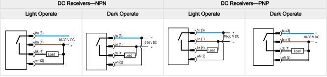
Cabled wiring diagrams are functionally identical.
